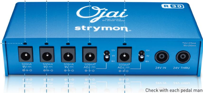
Check with each pedal manufacturer for recommended voltage, polarity, and required current. If a pedal requires more than 9, 12 or 18, please find details on those configurations here: [strymon.net/support/ojai-r30](http://strymon.net/support/ojai-r30)
